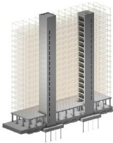
Cast-In-Place Reinforced Concrete Structure
